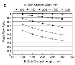
**Fig. 6.** Simulation of mass flow with different main channel width and branch channel length (a) straight branch channel width 30  $\mu$ m, (b) straight branch channel width 40  $\mu$ m and (c) straight branch channel width 50  $\mu$ m.
