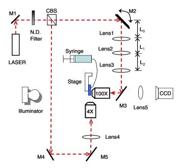
Fig. 2. Schematic diagram of the system setup.
