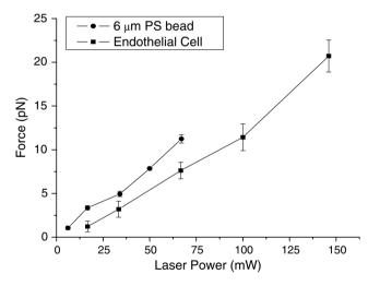
Fig. 12. Correlation between laser power and dragging force.
