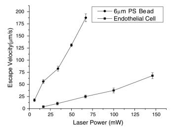
$\textbf{Fig. 11.} \ \ \text{Correlation between laser power and escape velocity}.$
