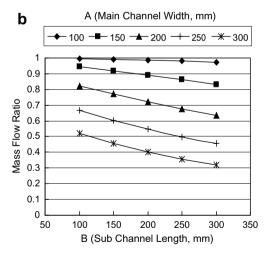
Fig. 5. Simulation of mass flow with different main channel width and branch channel length (a) nozzle-like branch channel width 20  $\mu m$  and (b) nozzle-like branch channel width 30  $\mu m$ .
