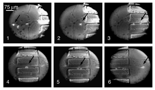
(a) a 6µ m polystyrene bead (see the solid arrow) is guided from main channel into construction area through branch channel.
