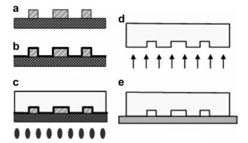
**Fig. 7.** Fabrication sequence of micro channel. (a) Pattern the geometry of micro channel by photo resist, (b) deposit Teflon, (c) pour PDMS on the wafer and heat it, (d) O<sub>2</sub> plasma treatment and (e) Bonding with glass.
